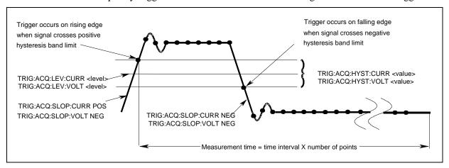
Figure 7-5. Commands Used to Control Measurement Triggers
